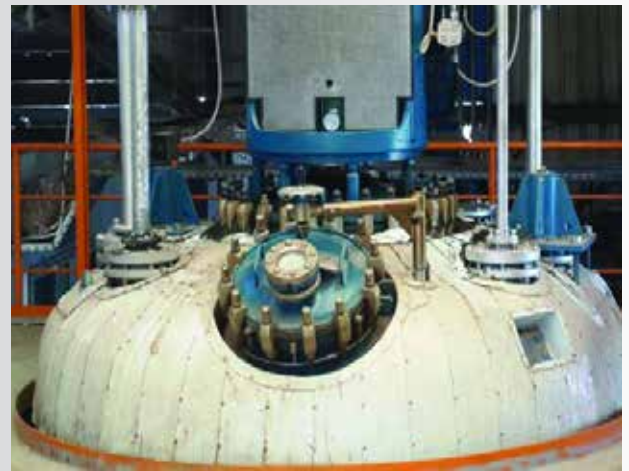
2 nd generation concrete admixtures main raw material, Sulphonated Naphthalene Formaldehyde (SNF) polymers, production in Jordan
